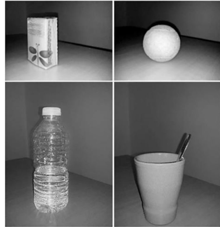
Fig 1. Objects used to assess grasping. Half-filled water bottle (height 22 cm, upper diameter 3 cm and lower diameter 6 cm, weight 260 grams); Teaspoon (length 14 cm, thickness 1 mm, weight 90 grams), Packet of paper tissues (height 7.5 cm, length 5 cm, thickness 2.5 cm, weight 20 grams) and Tennis ball (diameter 6 cm, weight 58 grams).
